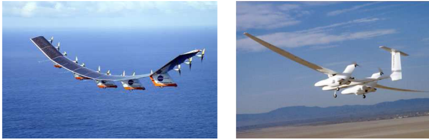
Fig. 1 Aerovironment's Helios (left) and Aurora Flight Sciences' Theseus (right) showing large wing deflections (Courtesy NASA Dryden).
