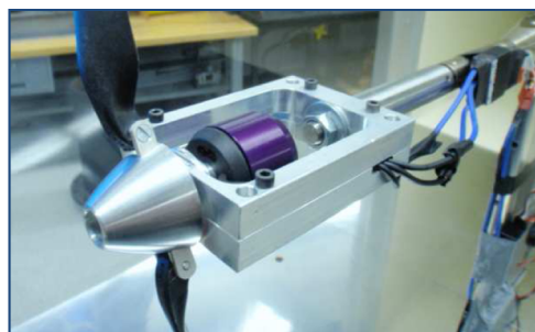
Fig. 17 2-ft-by-2-ft wind tunnel test setup for calibration of the propulsion assembly.
